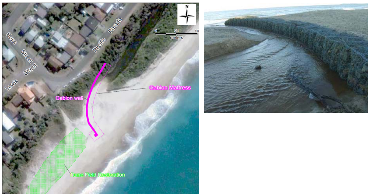
Figure 3: Design of the training wall that was constructed at Racecourse Creek to control entrance migration south (left) (from Worley Parsons, 2010a). Note how the training wall
