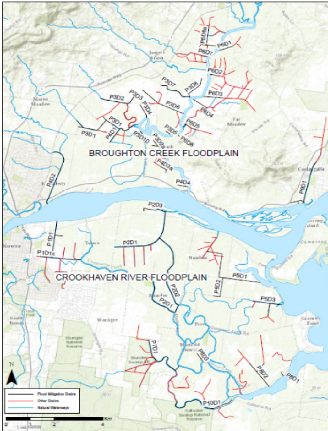
Figure 1. Location of major flood mitigation sub-catchments in Broughton Creek and Crookhaven River.
