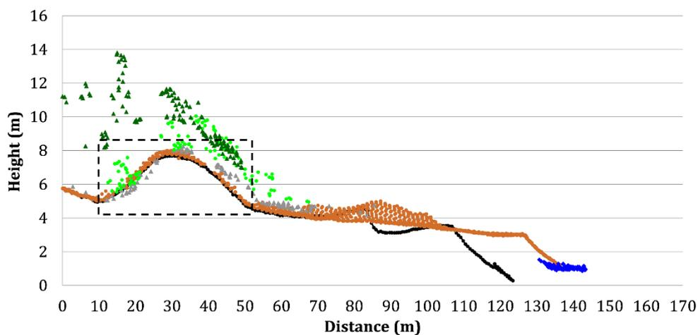
**Figure 6. a) On-site vegetation survey of Werri foredune, noting vegetation height, structure and dominant species present. b) The same profile geographically, but generated using the airborne LiDAR. Note the similarity in vegetation height, structure and extent, as well as the foredune morphology between the LiDAR profile and RTK GPS (black inset) (Data Source: LPI [2011]).**
