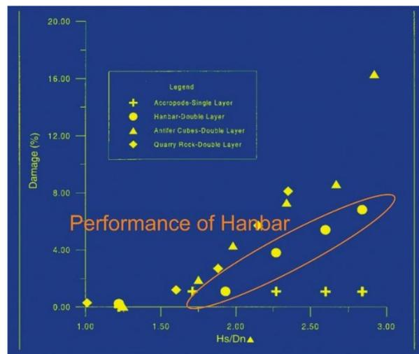
Figure 10a MHL physical modelling comparing Accropode, rock, Antifer cubes and Hanbars (MHL 1997)
