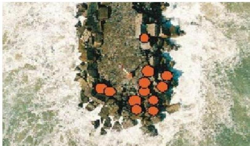
Figure 10b Coffs Harbour east breakwater head indicating locations of 40t concrete blocks displaced in the May 1997 storm
