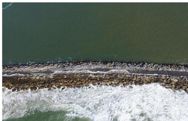
**Figure 5b Clarence north training wall crest damage post-June 2016 storm
