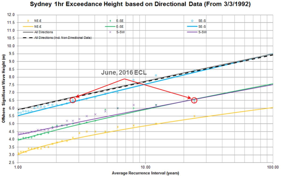
**Figure 3 1-hr ARI based on the Sydney offshore buoy based on directional wave measurement**
