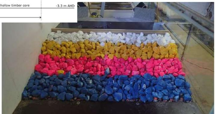
Rubble Mound Seawall: Section and Testing (WRL, 2016)
